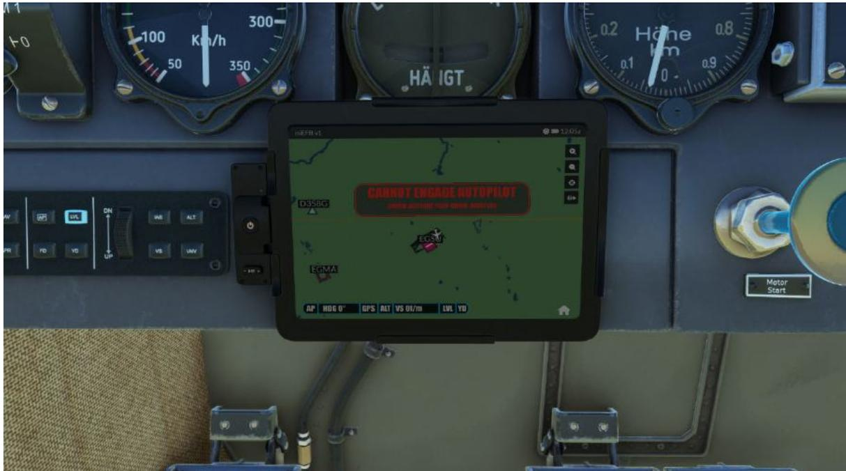
If the conditions for AP functions are not met, i.e. gear down, flaps down, speed, altitude, vertical climb/descent, Etc. a warning box will pop-up on the EFB telling you why that function cannot be engaged.
