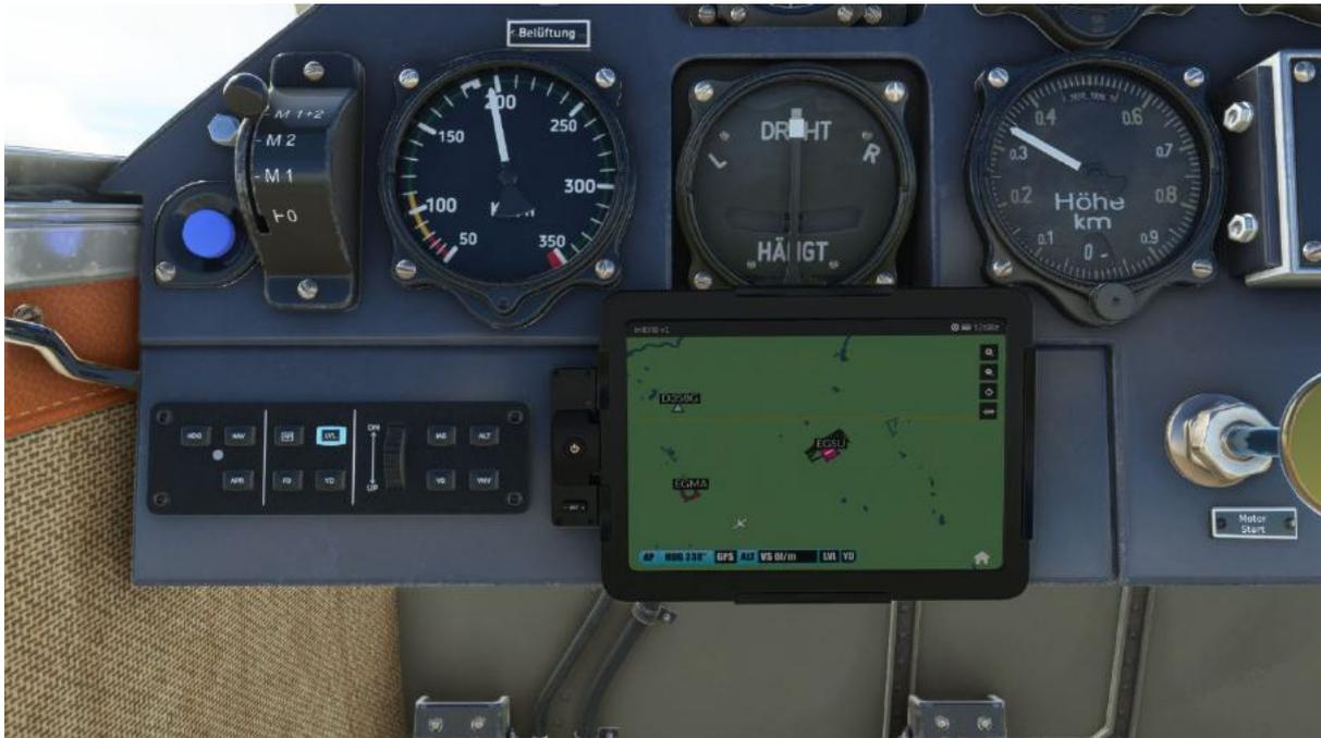
When an AP function is enabled the button in the control panel will highlight blue and the AP status bar on the bottom of the map page will also indicate which mode is "ON". In this example we have **AP**, Heading (**HDG**) and Altitude (**ALT**) hold on.
