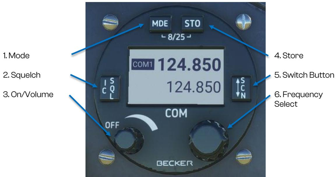
The main display shows the communications channel selected, the main frequency and the standby frequency.
