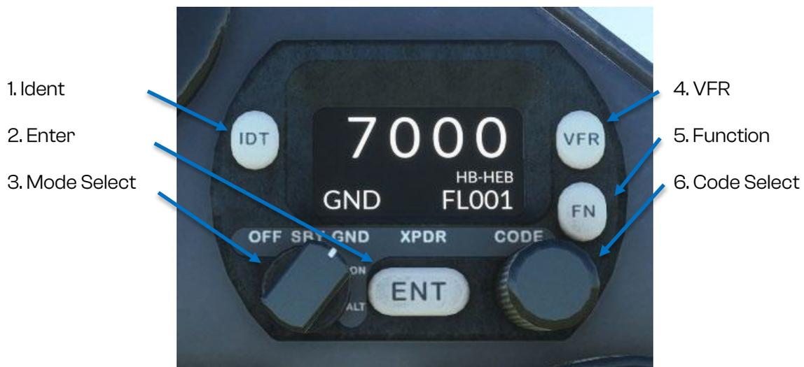
The main display shows the operating mode of the transponder, the reported pressure altitude, and the current squawk code and Flight ID.
