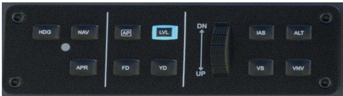
**HDG:** Heading hold mode locks the current heading and that value is updated each time this mode is activated. You can manually turn the plane whilst in HDG mode and press the button again to set current heading.
