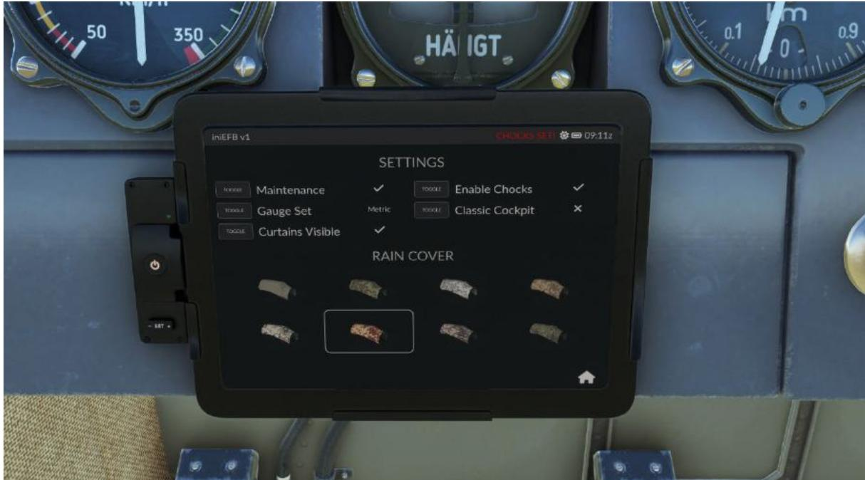
To enable the use of chocks, go to the Settings page and Tick Enable Chocks. The chocks will display in the external camera view and a warning will come up on the EFB top section and in addition a red warning will pop up "Chocks Set".
